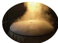
Rice washing machines are used to rinse when making standard sake, on the other hand, the highly polished rice for Ginjo-shu is still rinsed by hand delicately. The rice is then steamed, making it easier for the enzymes in Koji-mold (*Aspergillus oryzae*) to break down the starches. At mass producing sake breweries, all of the processes from washing to steaming(for standard sake) are done by automated machines.
